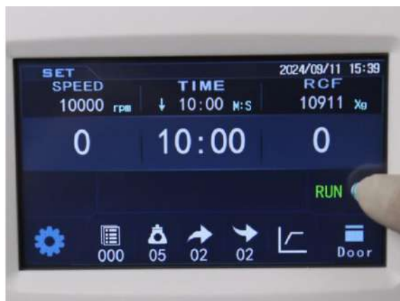
Glove-sensitive LCD touch screen with password protection for parameter setting
